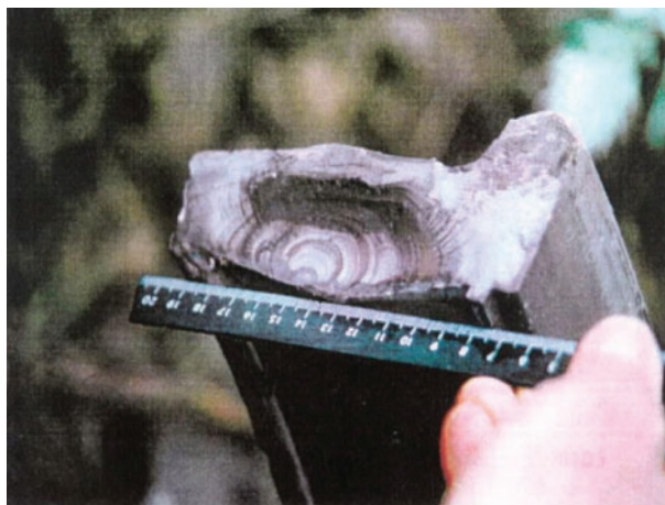
9 The failed tyre (rim) of the Eschede wheel. The fatigue crack is self evident
