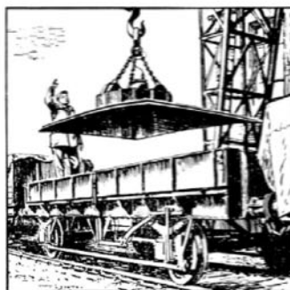
Here we show steel plate being unloaded by magnetised grab.
